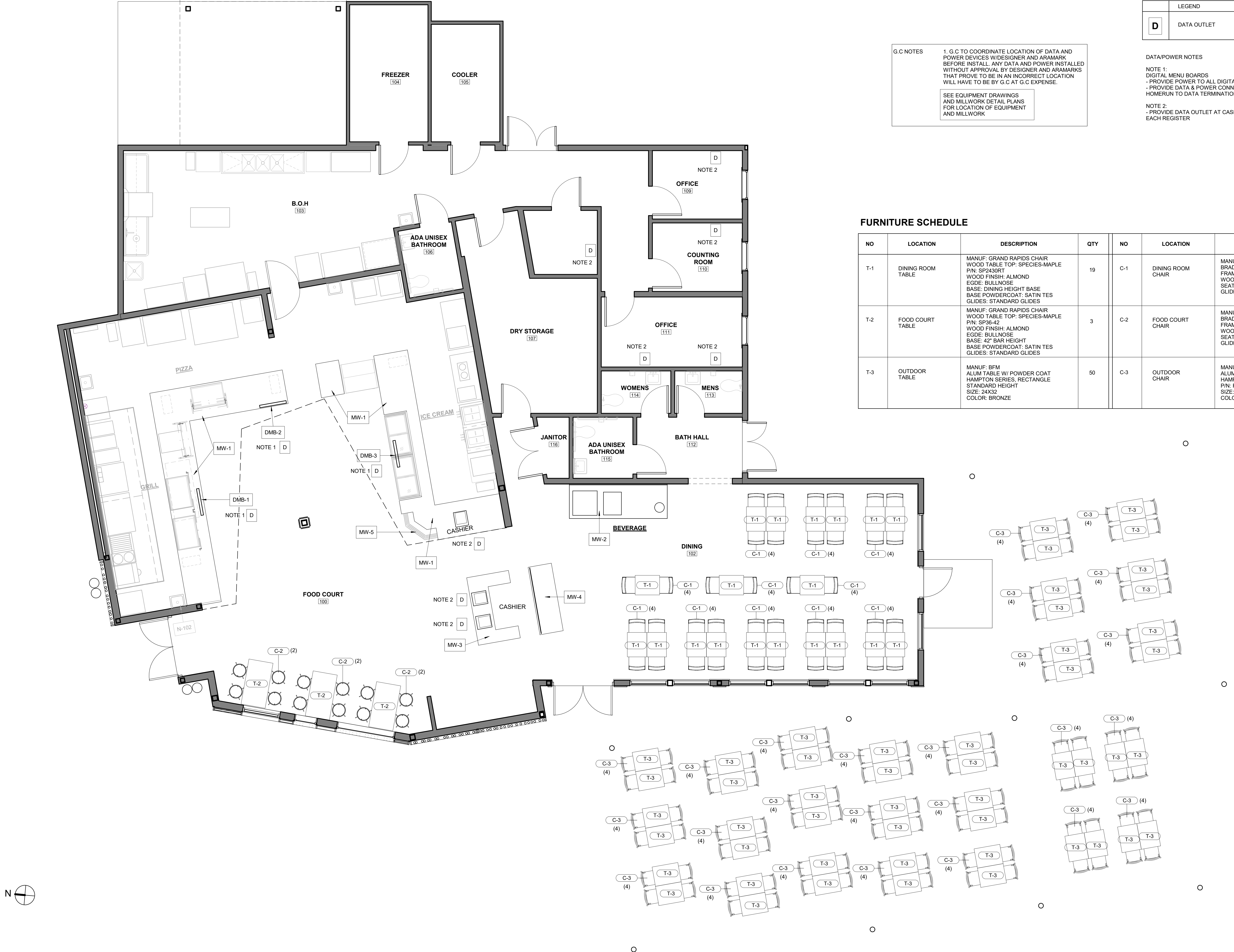
1 FIRST FLOOR MILLWORK AND FURNITURE PLAN 1/4" = 1'-0"
