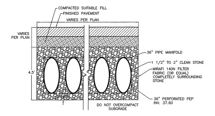
PEP = HIGH DENSITY POLYETHYLENE PIPE BY HANCOR, ADS OR EQUAL
