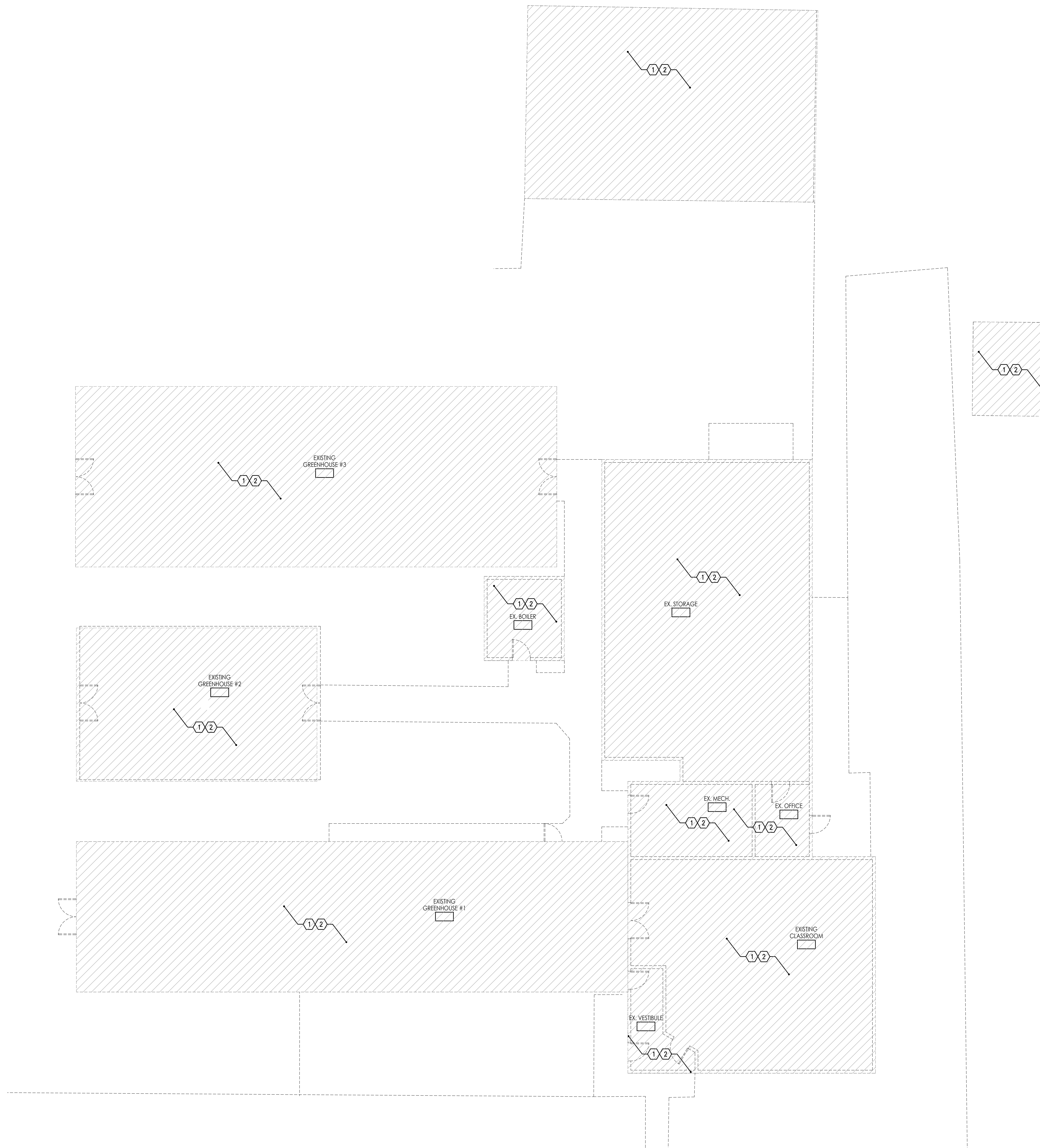
1 H101 MECHANICAL - DEMOLITION WORK - GREENHOUSE & ASSOCIATED BUILDINGS SCALE: 1/8" = 1'-0"
