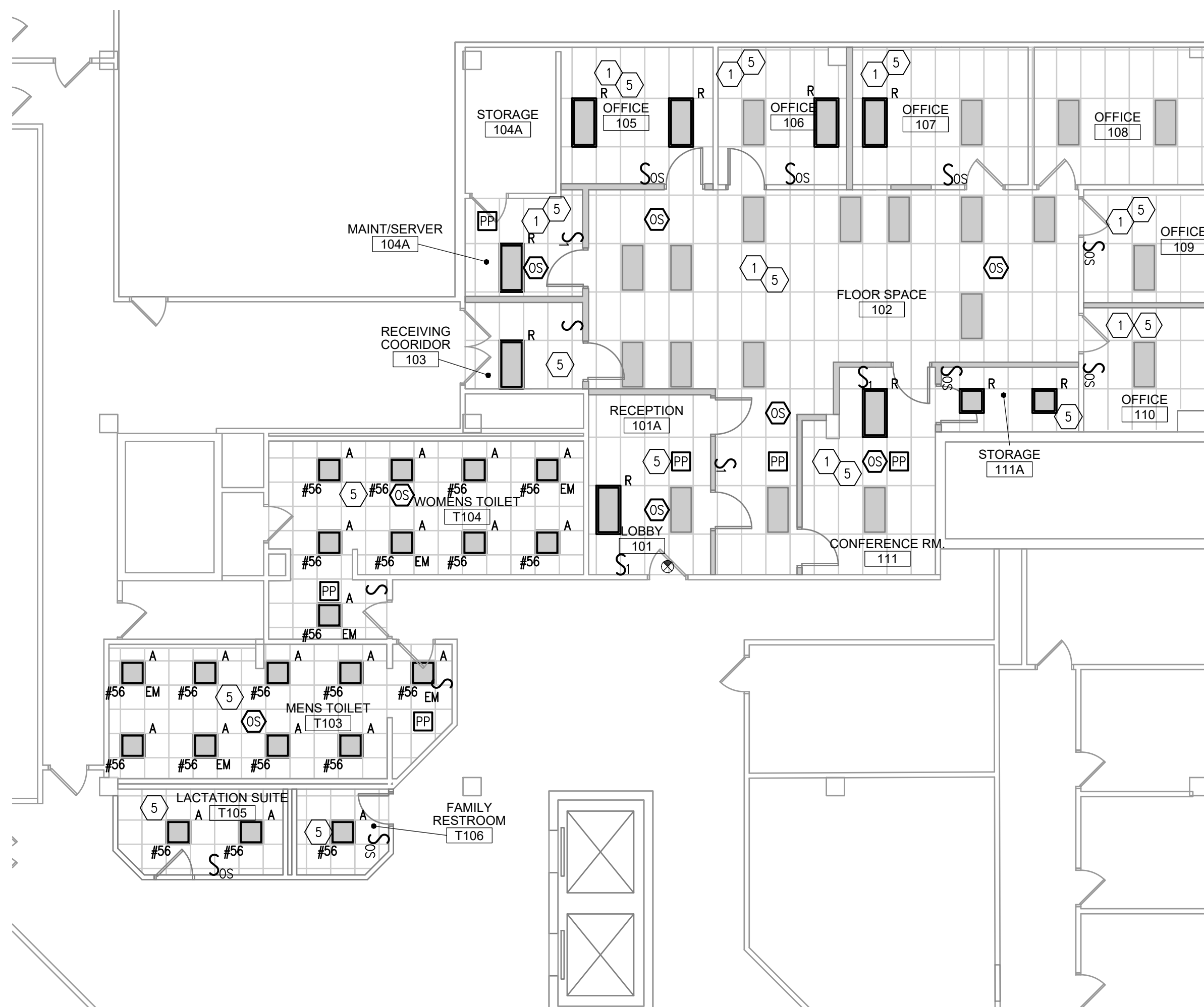
2 ELECTRICAL FIRST FLOOR AGING & DISABILITY LIGHTING PLAN 1/8" = 1'-0"
