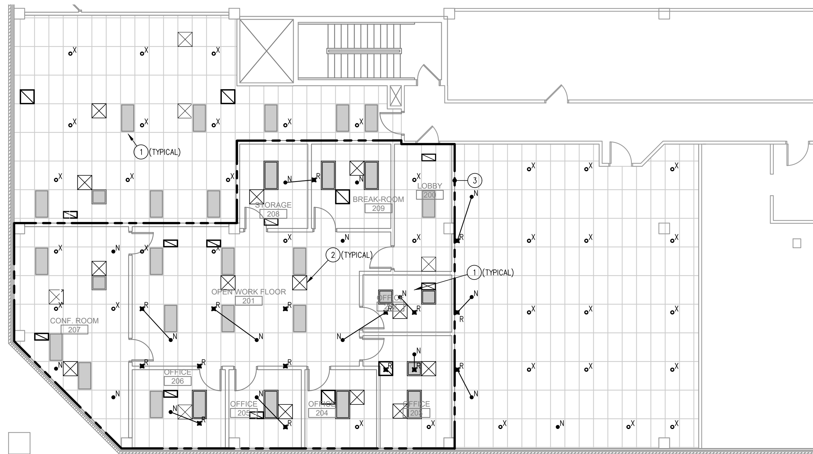
1 2ND FLOOR SPRINKLER HEAD RELOCATION PARTIAL PLAN 1/8" = 1'-0"
