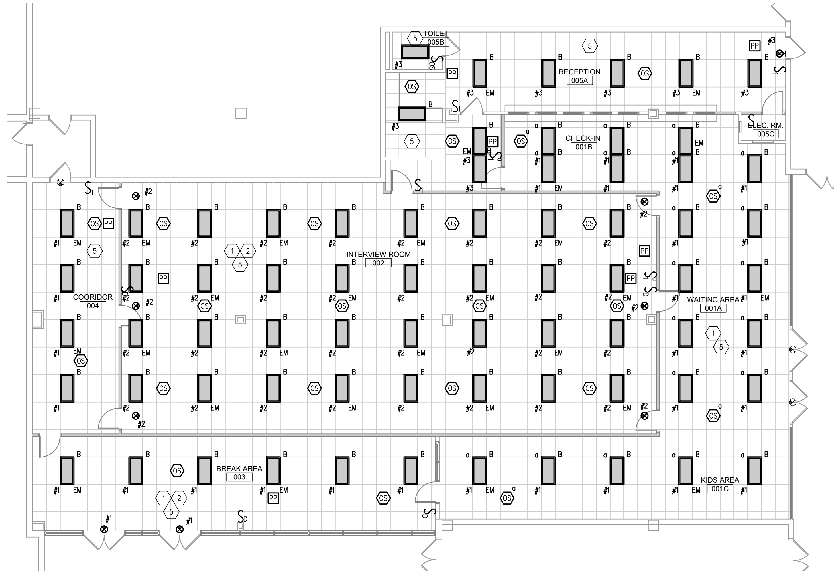
1 ELECTRICAL GROUND FLOOR INTERVIEW ROOM LIGHTING PLAN 1/8" = 1'-0"
